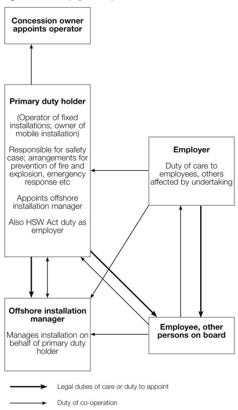
Figure 1 Offshore safety legislation: duty structure
