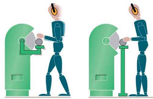
methods showing how the operator was isolated from the vibration
