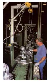
Suspended hand tool in use, showing support cable
