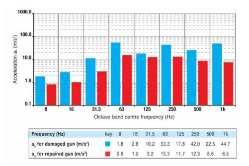
Vibration acceleration measured on a needle gun before and after it was repaired
