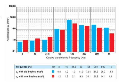
Vibration acceleration measured on a chainsaw before and after antivibration bush replacement
