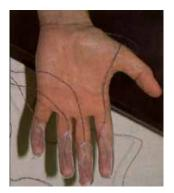
Hand fitted with thermocouples
