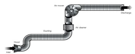
Figure 1 Common elements of a simple LEV system
