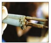
Figure 2 On-tool extraction soldering iron
